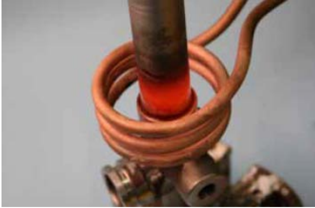
Fig. 2: Induction heating effect.
